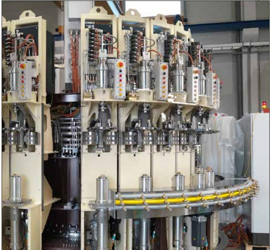
Autonomous sections; if a fault occurs, each segment of the blow moulding machine can be replaced in a maximum of ten minutes. That means a huge reduction in downtime.
