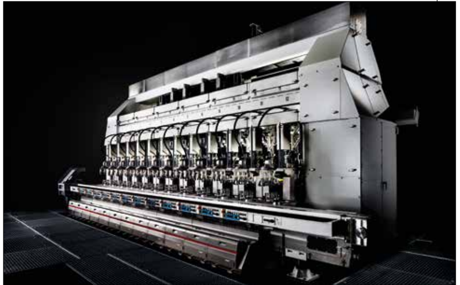
Modern glass production: Heye's SpeedLine IS machines promise high productivity and quality in container glass manufacturing – thanks not least to controls made by futronic.
